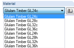
Figure 5.5: Selection of strength class for glued-laminated timber
