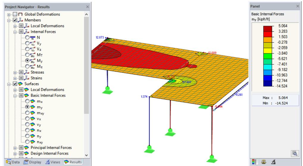
Figure 8.3: Setting internal forces of members and surfaces in *Results* navigator
