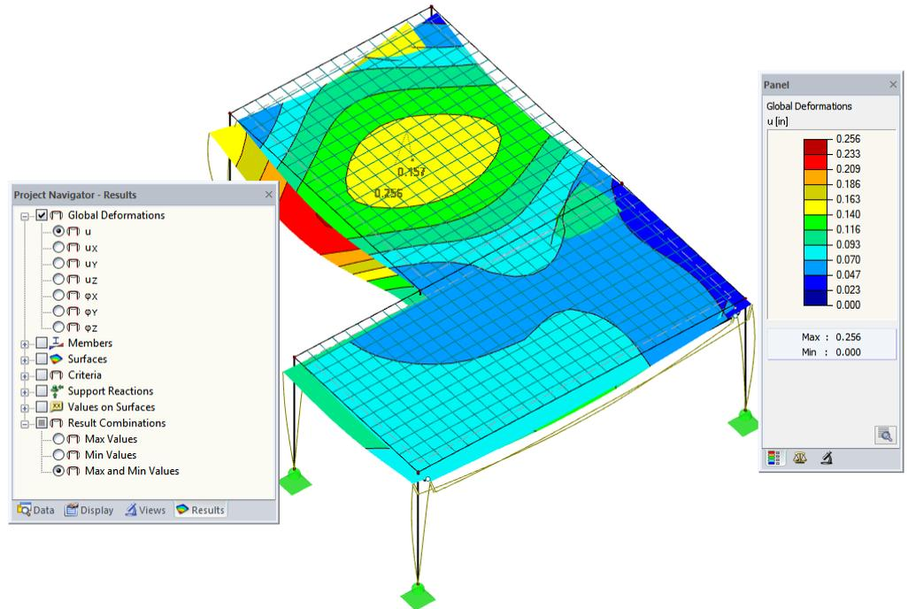
Figure 8.1: Graphic of max/min deformations for result combination RC1
