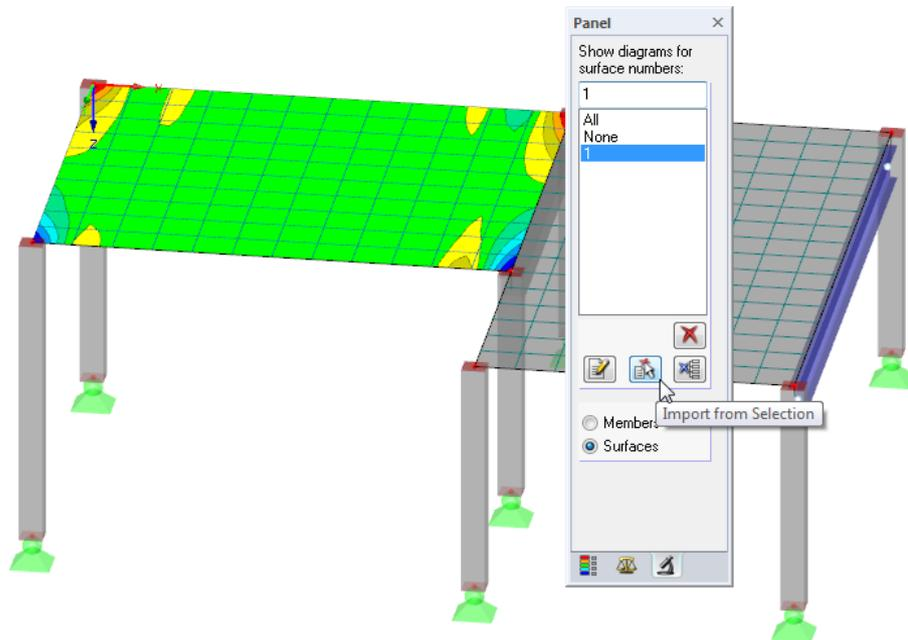
Figure 8.10: Shear force diagram of left surface
