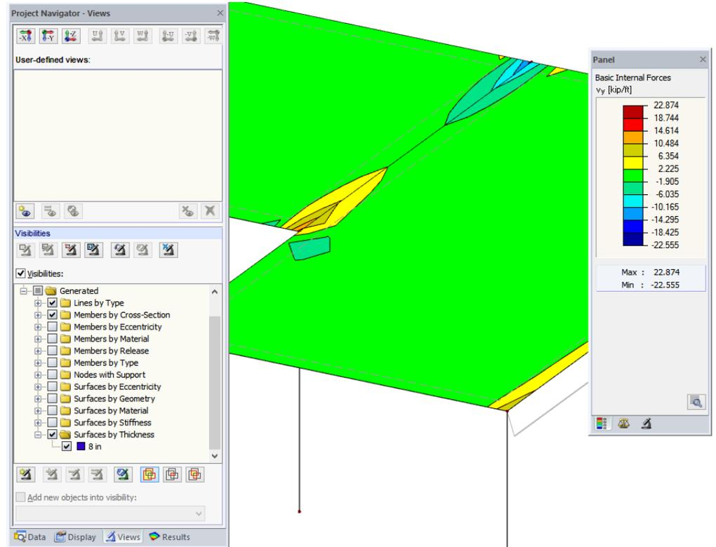
Figure 8.8: Shear forces of floor
