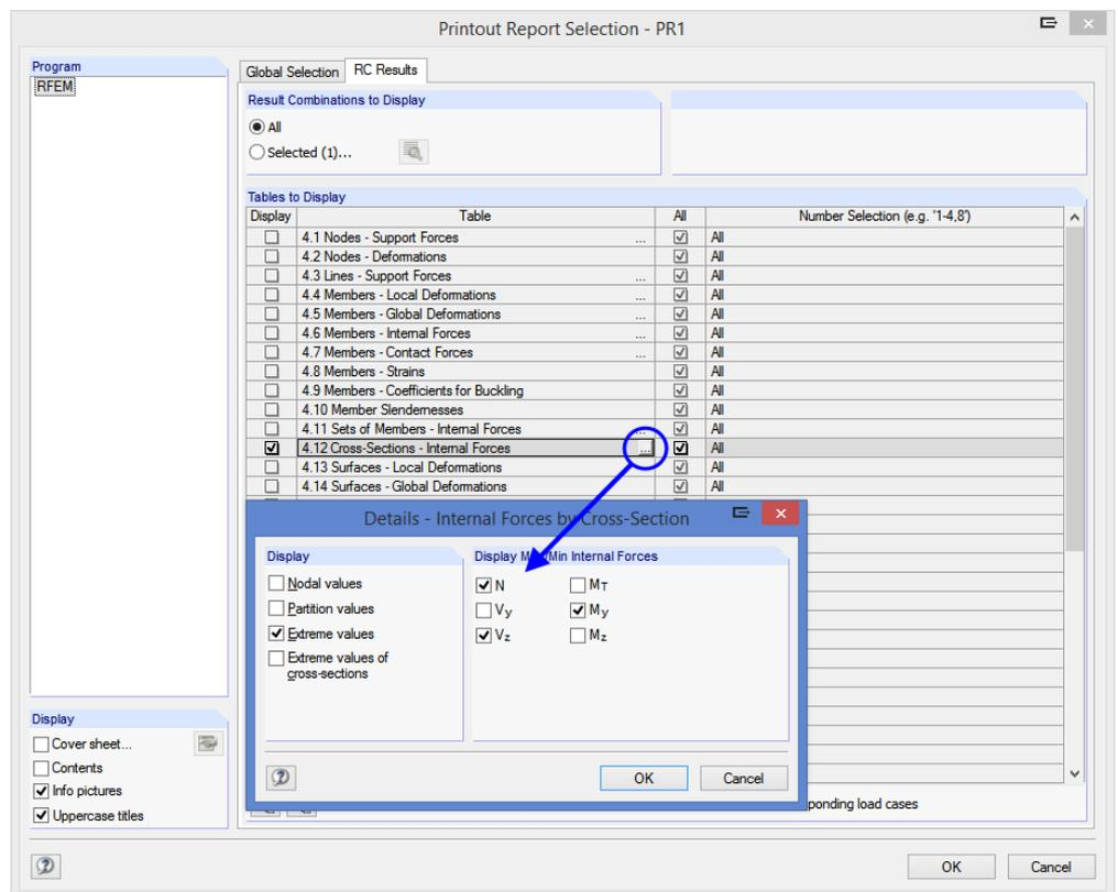
Figure 9.4: Reducing output of internal forces by means of *Printout Report Selection*
