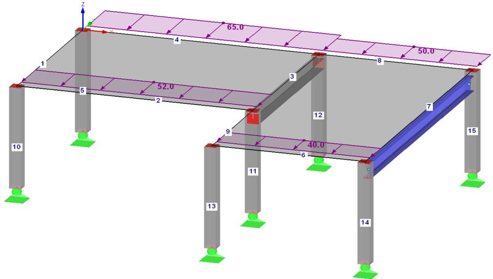
Figure 5.13: Graphical input of wind loads
