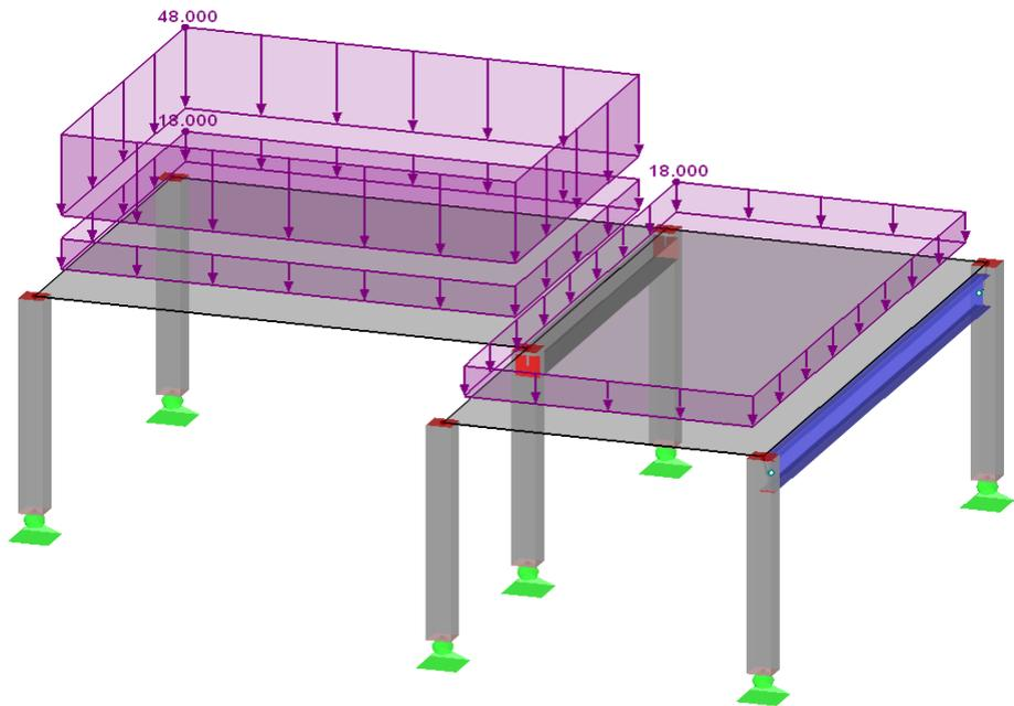
Figure 6.3: Loads of load combination CO1
