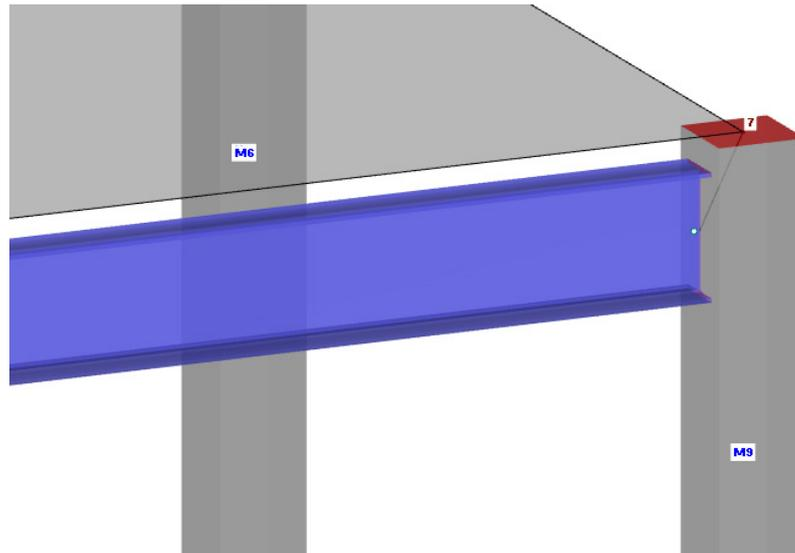
Figure 4.25: Steel girder with release and eccentricity
