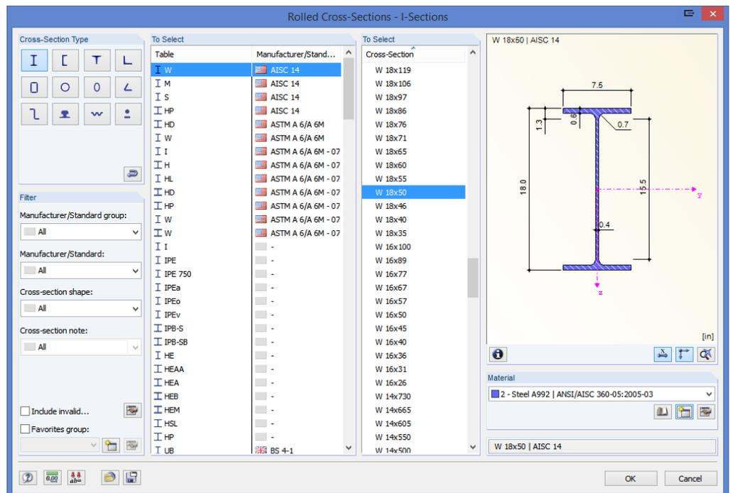
Figure 4.8: Dialog box *Rolled Cross-Sections - I-Sections*
