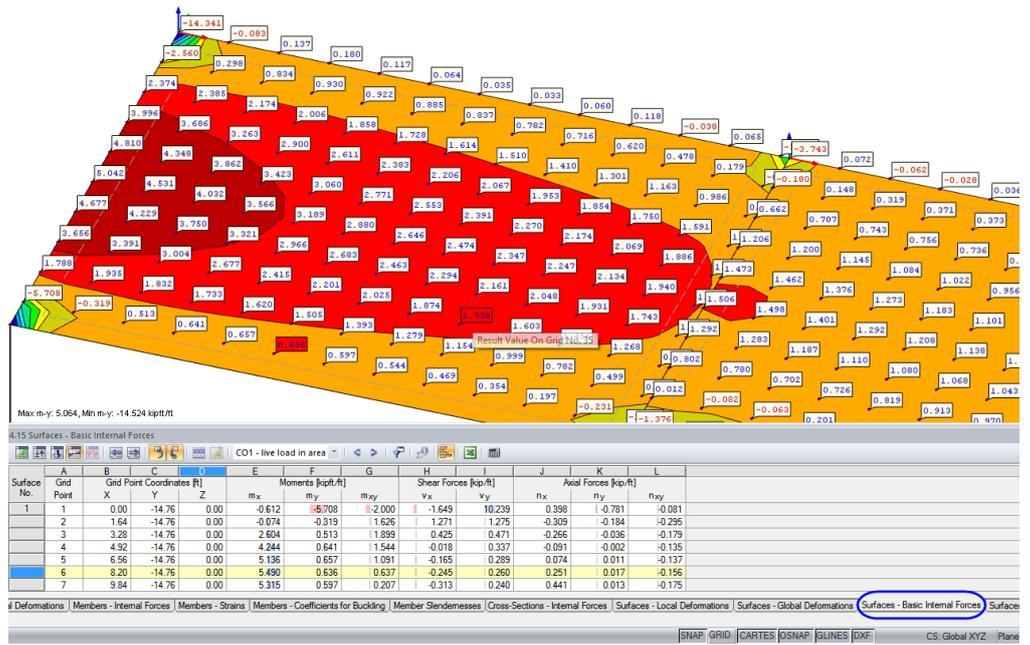
Figure 8.6: Surface internal forces in Table 4.15 and marker of current grid point in the model
