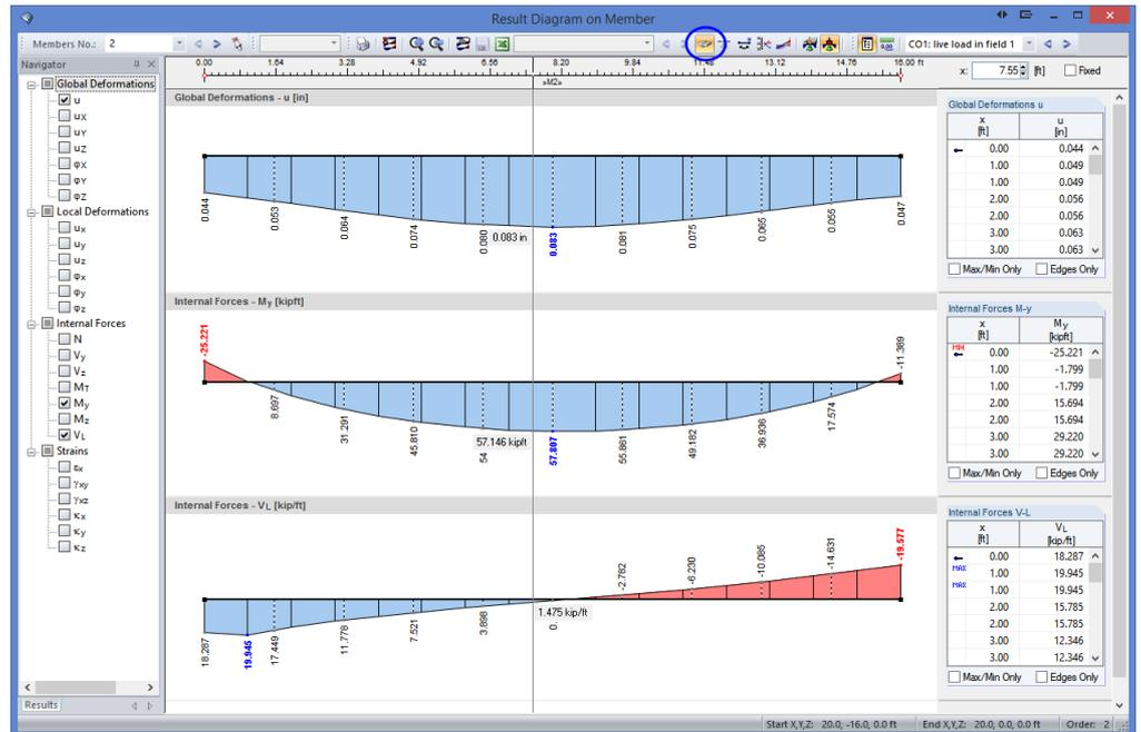
Figure 8.11: Display of result diagrams of downstand beam
