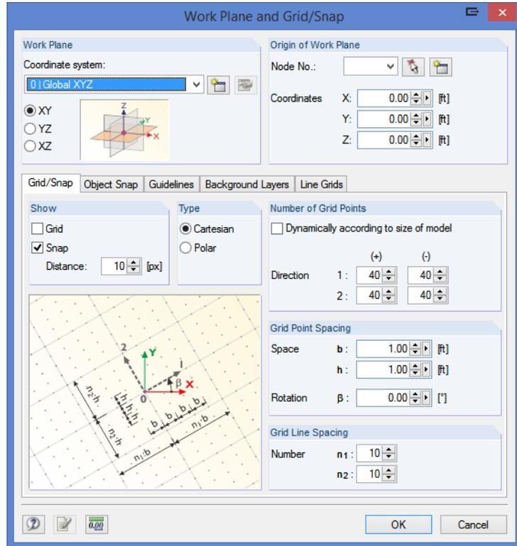
Figure 4.1: Dialog box *Work Plane and Grid/Snap*
