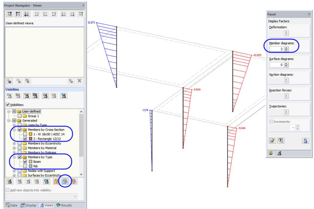
Figure 8.7: Moments  $M_y$  of concrete columns in scaled representation
