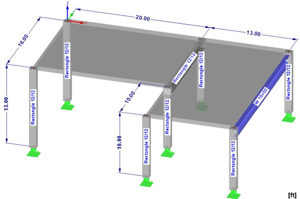
Figure 2.1: Structural system
