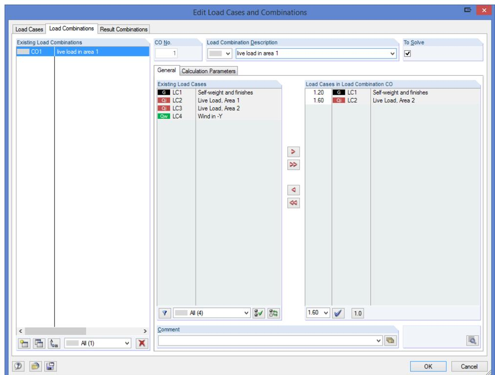
Figure 6.1: Dialog box *Edit Load Cases and Combinations*, tab *Load Combinations*
