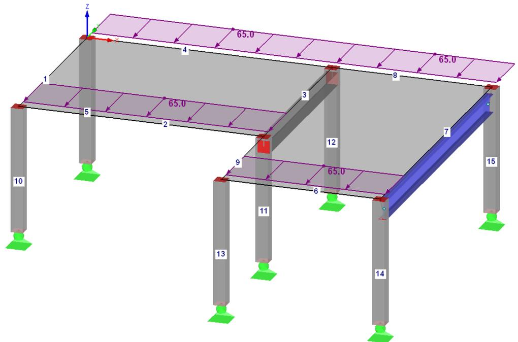
Figure 5.12: Graphical input of wind loads without adjustments
