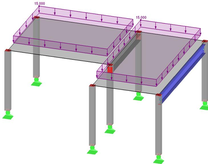
Figure 5.4: Graphical input of floor load
