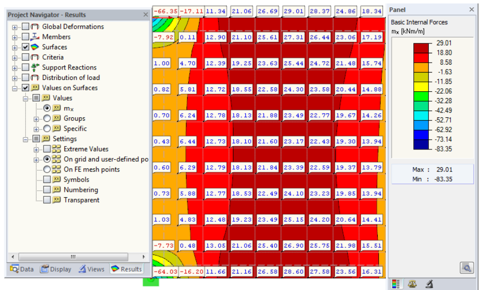
Figure 8.4: Grid point moments m_x of floor slab in Z-view (CO1)
