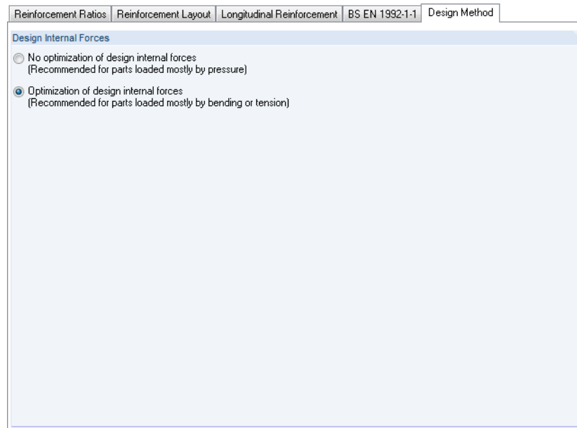
Figure 3.40: Window 1.4 Reinforcement, tab Design Method
