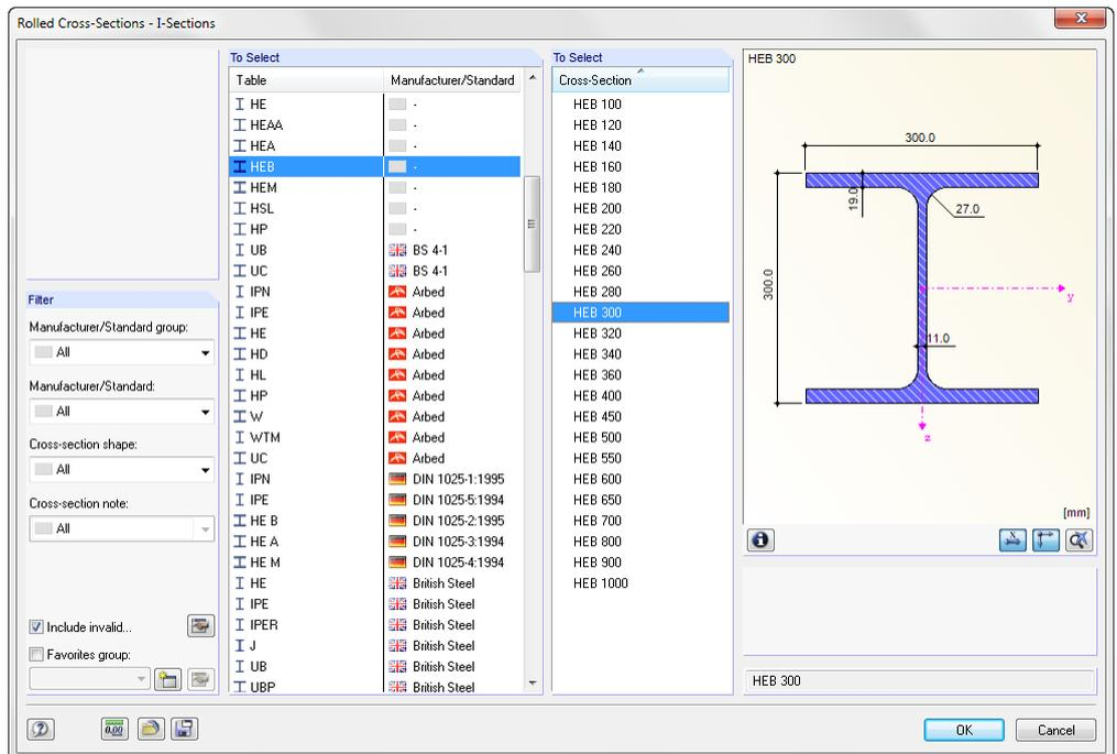
Figure 2.16: Cross-section library for *Rolled sections*
