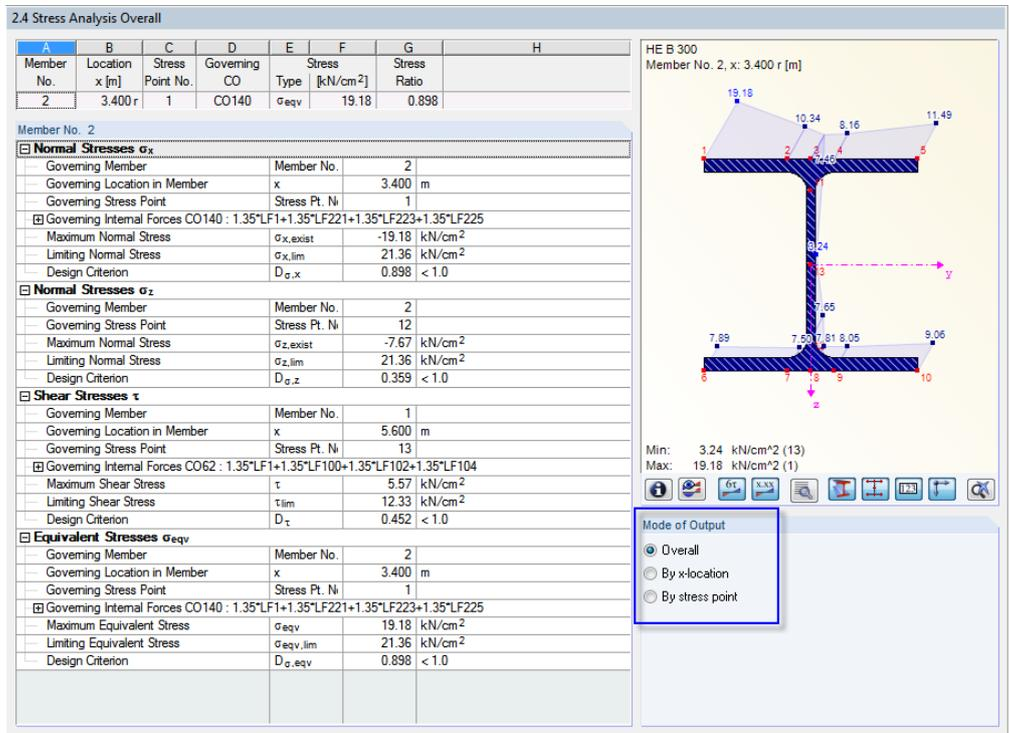
Figure 4.8: Window 2.4 Stress Analysis Overall
