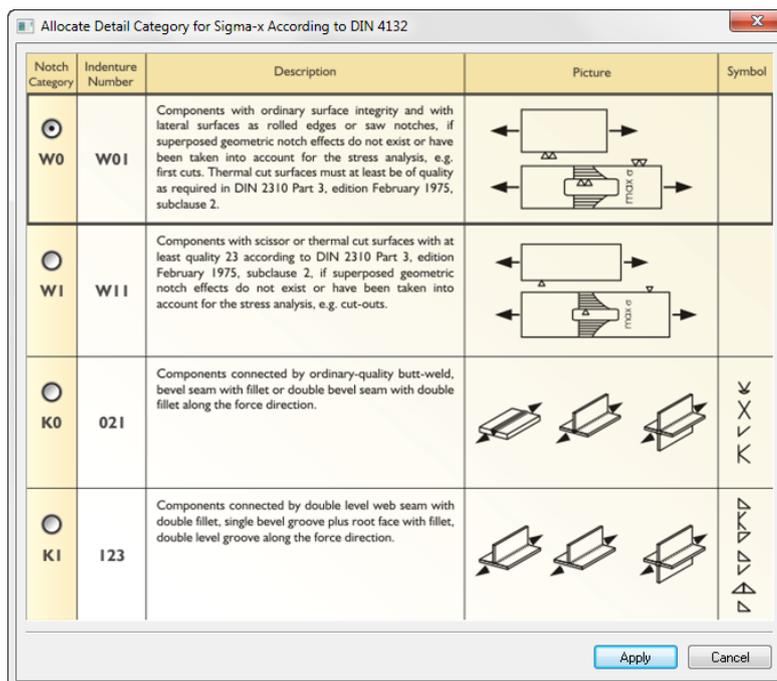
Figure 2.29: Dialog box *Allocate Detail Category according to DIN 4132*
