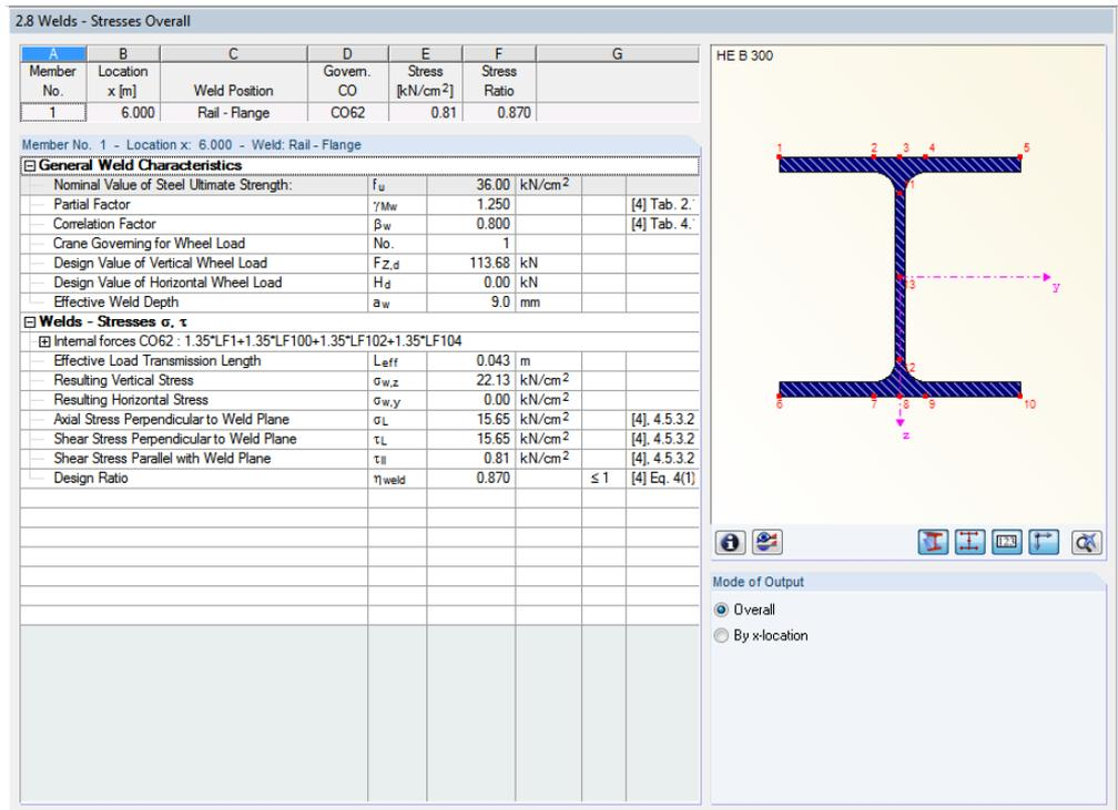
Figure 4.23: Window 2.8 *Welds - Stresses Overall*
