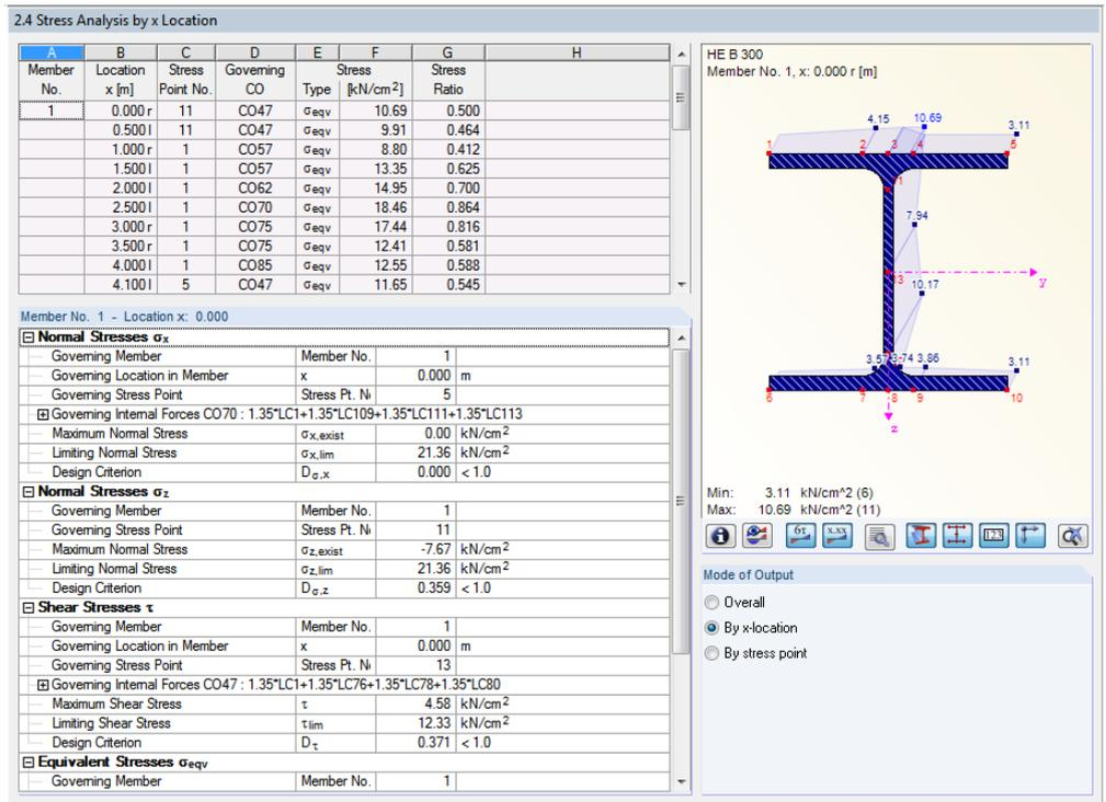
Figure 4.9: Window 2.4 Stress Analysis by x-Location
