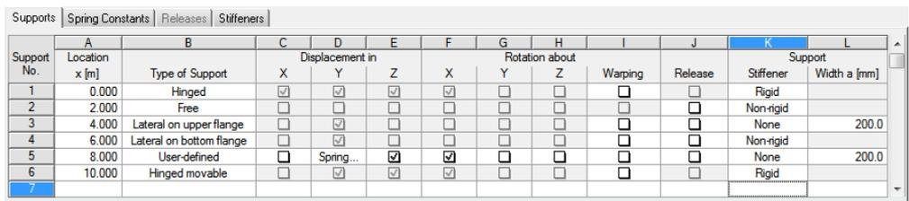
Figure 2.7 Window 1.2 Geometry, tab Supports
