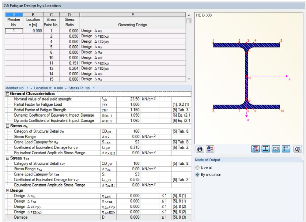
Figure 4.18: Window 2.6 Fatigue Design by x-Location
