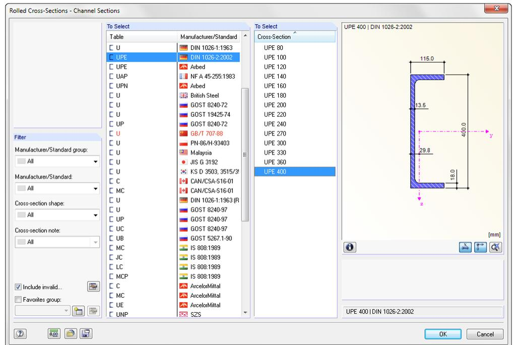
Figure 2.21: Cross-section library for *Rolled Cross-Sections - Channel Sections*
