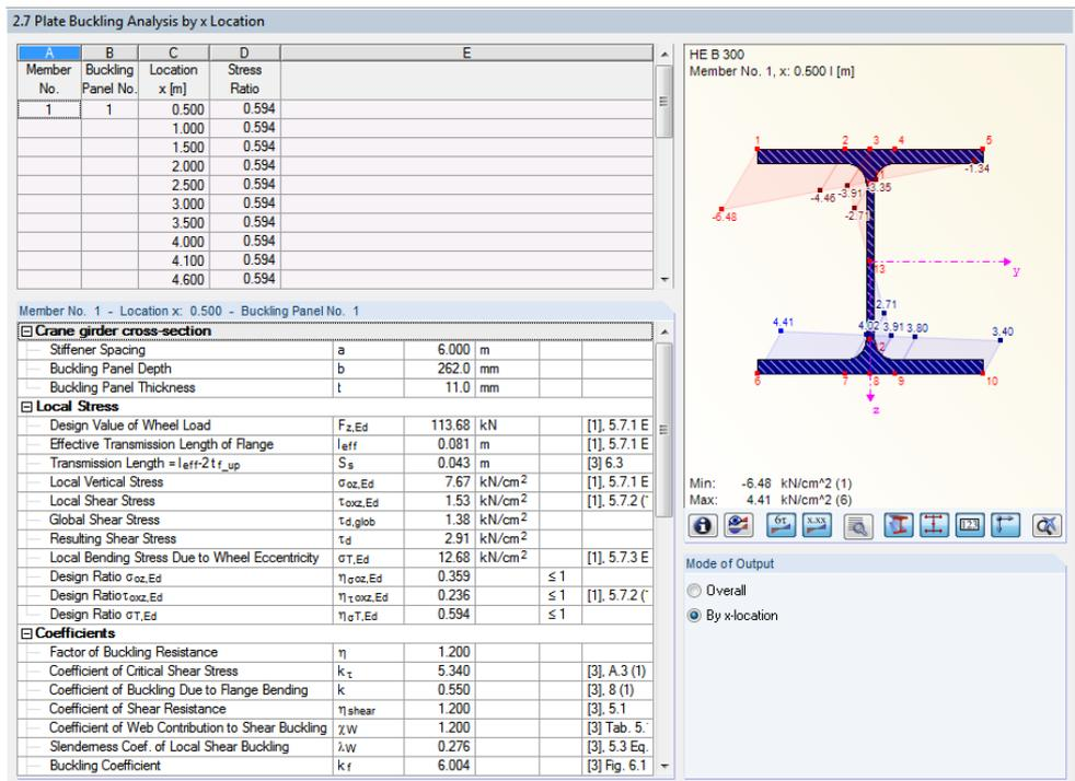
Figure 4.22: Window 2.7 Plate Buckling Analysis by x-Location
