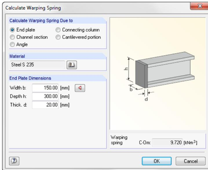
Figure 2.9: Dialog box *Calculate Warping Spring*
