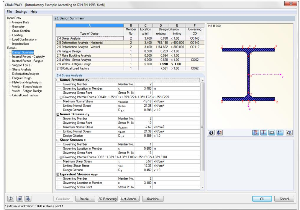
Figure 4.1: Results window with designs and results details
