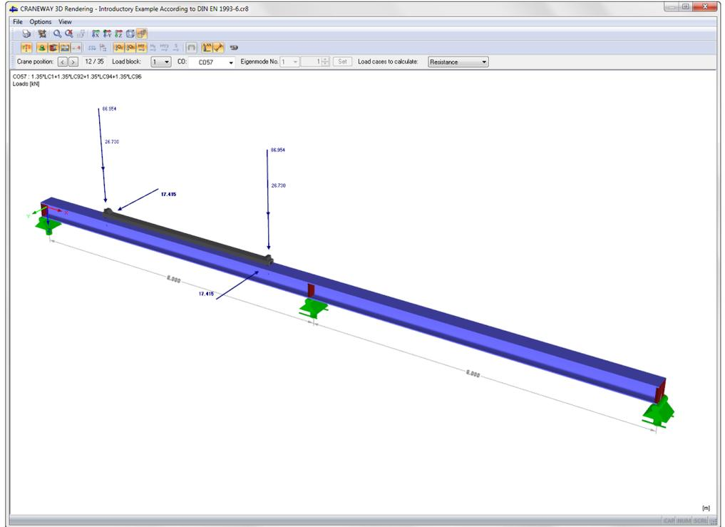
Figure 6.5: Graphic of the crane runway girder
