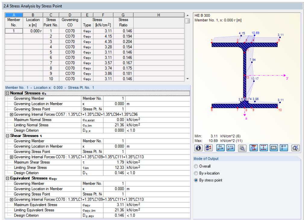
Figure 4.10: Window 2.4 Stress Analysis by Stress Point
