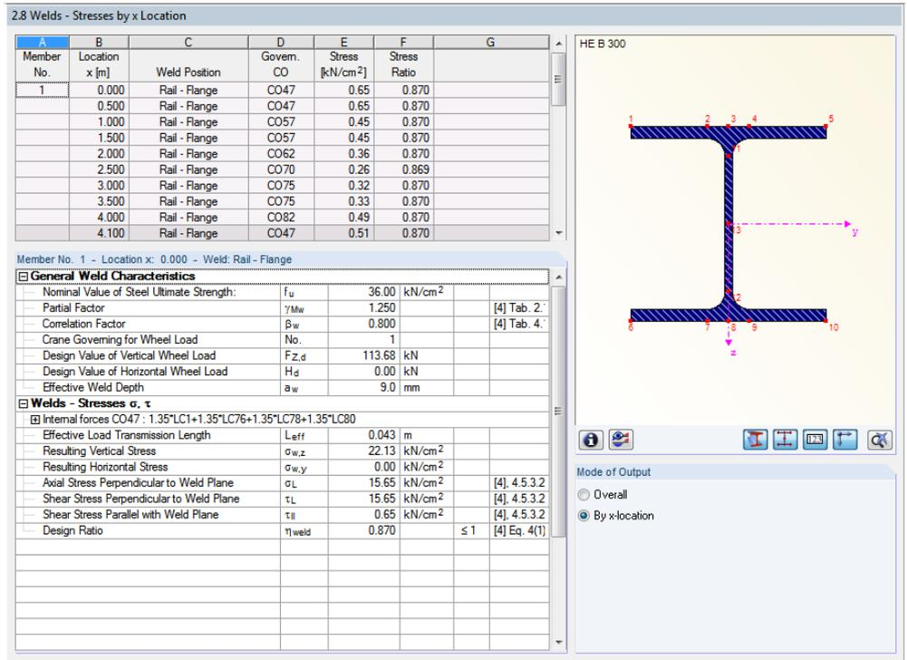
Figure 4.24: Window 2.8 *Welds - Stresses by x-Location*
