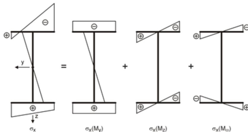
Figure 4.14: Normal stress components for biaxial bending with warping torsion
