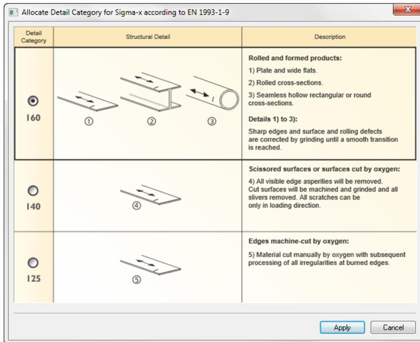
Figure 2.28: Dialog box *Allocate Detail Category according to EN 1993-1-9*
