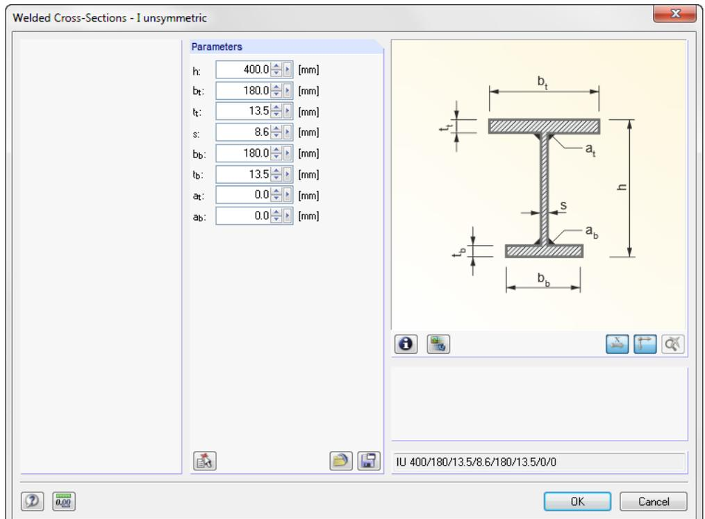
Figure 2.17: Parametric input for *Welded sections*
