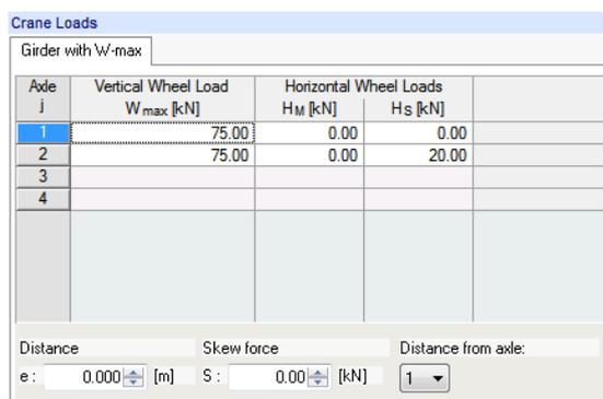
Figure 2.39: Section *Crane Loads* according to DIN 4132
