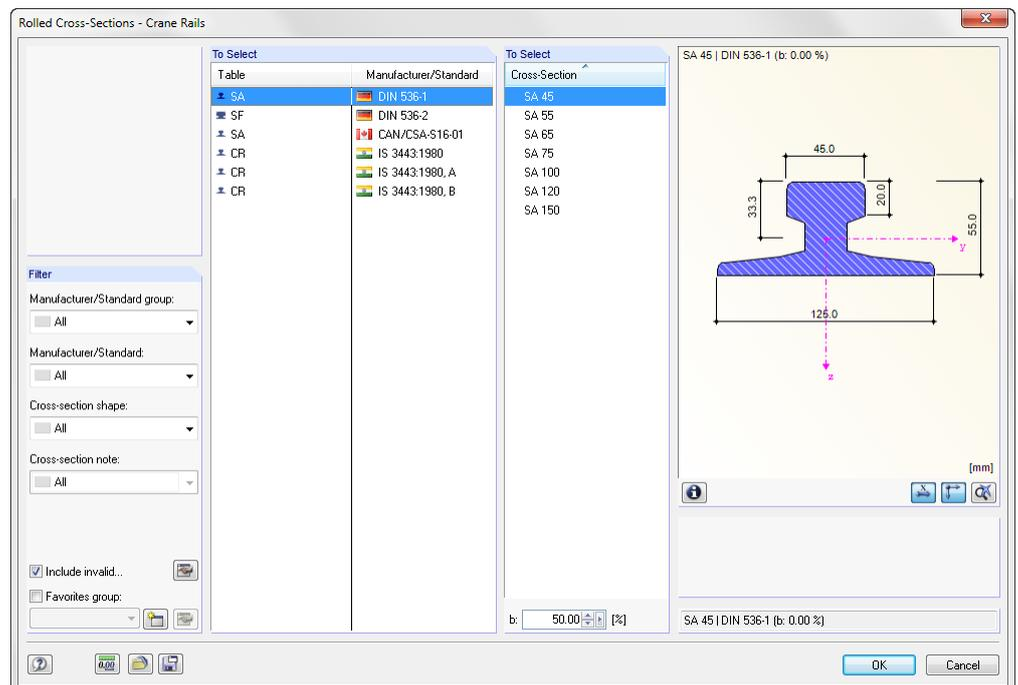
Figure 2.19: Cross-section library for *Rolled Cross-Sections - Crane Rails*
