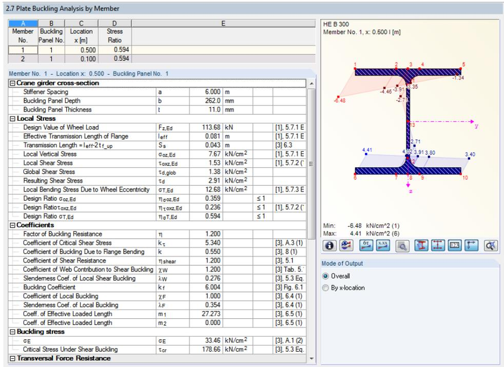
Figure 4.21: Window 2.7 Plate Buckling Analysis - Overall
