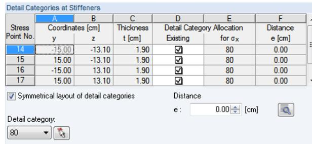
Figure 2.30: Section *Notch Categories at Stiffeners* for *Symmetrical layout of notch categories*
