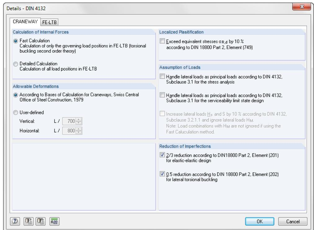
Figure 3.2: Dialog box *Details*, tab *CRANEWAY* for DIN 4132
