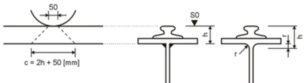
Figure 4.11: Length of the uniformly distributed wheel load
