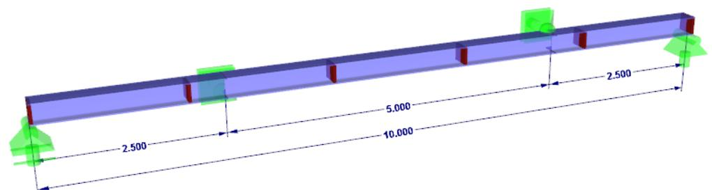
Figure 2.13: Regular positioning of the stiffeners only between the supports acting in the Z-direction
