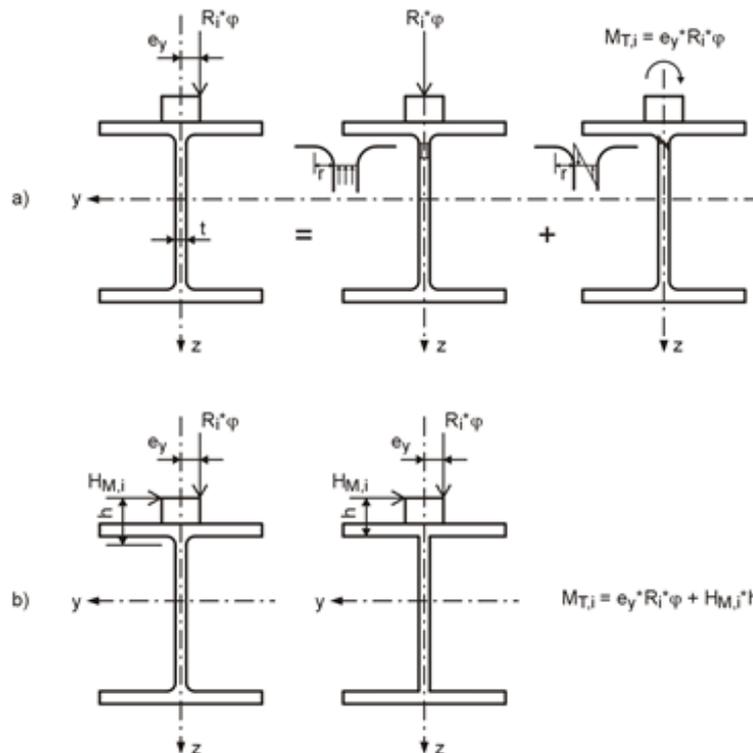
Figure 4.19: Stress at the upper edge of the web due to eccentric wheel load
